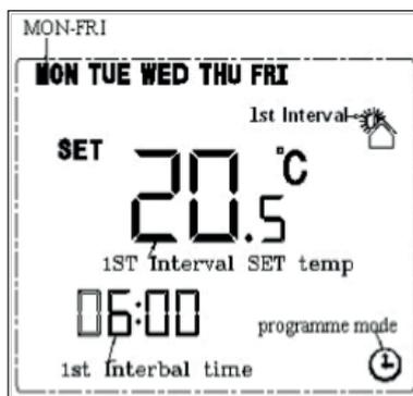
This planning allows you to set, for each of the six time-bands, the start time and the temperature setting of the same band of the day or week (not the end time). The thermostat's factory settings for following the programme 5+2 (MON-FRI, SAT-ONN): the 6 hour bands configurable are shown by the symbols indicated on the side.
