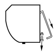
Unscrew the mounting plate and remove it.
