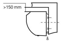
Install the air curtain on the mounting plate, making sure that it is in the safety position and tighten it with the appropriate screws.
