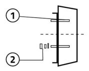
Drill a hole as shown in the instructions and insert the screw into it, securing it in the cement.
