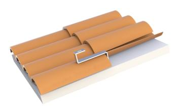
Fixing of photovoltaic systems on roofing tiles supported by strips of varying thickness.
