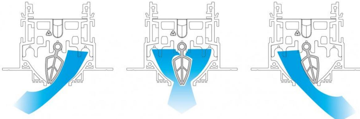
DIAGRAMM DER HORIZONTALEN LUFTSTRÖME MIT GENEIGTER STÖRKLAPPE
