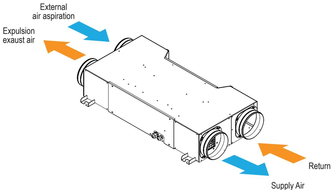
It is important that the fresh air is drawn in from outside the building and that the exhaust air is expelled outside. Furthermore, it is advisable to install protective grilles for the pipes on the outside. When making the first connection of the ventilation system, it is necessary to refer to the electrical panel on the machine.
