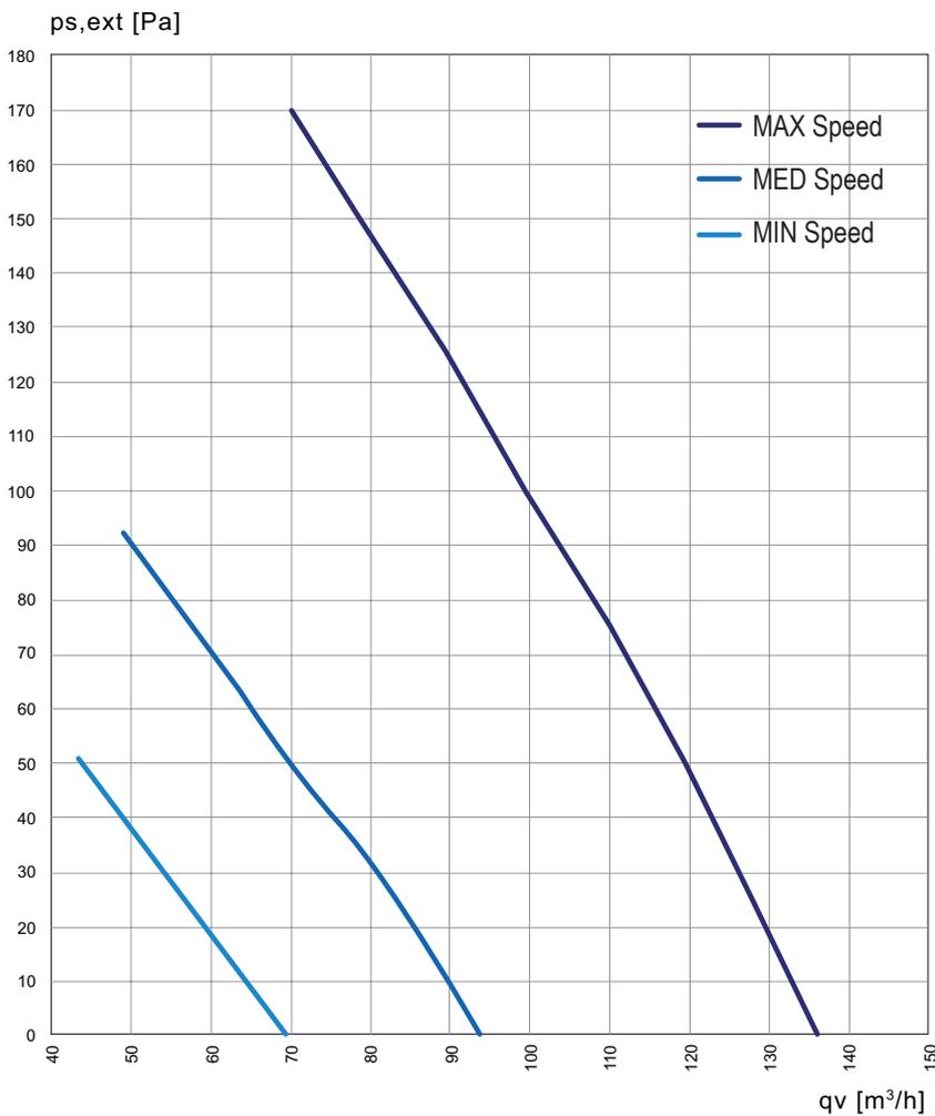
The reported static head must be considered useful for the ducts, considering a unit equipped with G4 filters on the delivery side.
