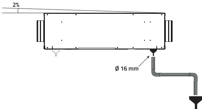
Condensation may form during normal machine operation. It is necessary for this condensate to leave the recovery unit to avoid stagnation problems. The appliance is therefore equipped with two condensate outlets and should be fixed with a 2% slope towards the side of the condensate drain pipe, connecting it to a water drain pipe (pipette connection Ø 16 mm).
