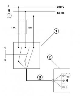
Omnipolar thermal magnetic protection switch compliant with EN 61508:1
