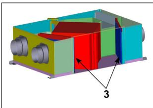
The filter structure at each inlet and outlet of the renewal air allows the filter to be removed from the side. Operating sequence:
