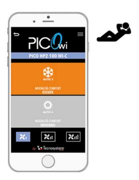
The system, set in Winter Comfort or Summer Comfort mode, is enabled, exploiting the temperature difference between the outdoor and indoor environment, in order to reach an ideal temperature in the indoor environment. You can choose between 3 available speeds.
