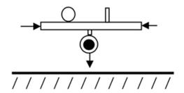
In order to ensure proper operation and maintain the longevity of the Regulator, it is recommended to install it with the outlet turned downwards.
