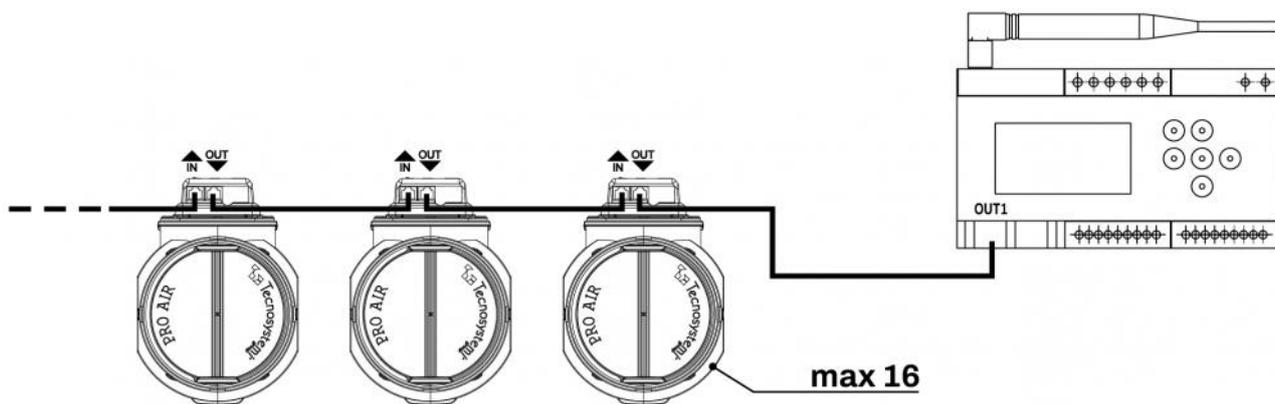
Up to 16 motorised dampers can be connected in a cascade.
