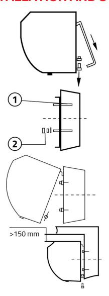
Unscrew the mounting plate and remove it.
