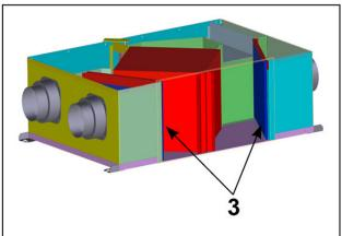
The filter structure at each inlet and outlet of the renewal air allows the filter to be removed from the side.
