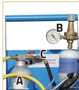
1. *Remove the aluminum container A from the support.*
